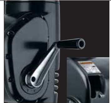
Manual operation switch and gear socket
