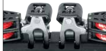
Toggles have a low pivot point to handle mainsheet loads up to 40 degrees from vertical, while allowing cars to roll freely.
